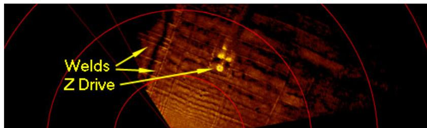
*Hull Scan of Barge*
