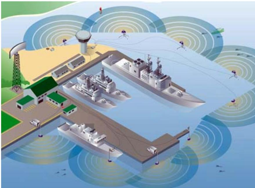
*Graphic view of navy vessels moored alongside a diver-detection system set up as a security perimeter around high-value assets to protect against enemy divers and submersibles.*
