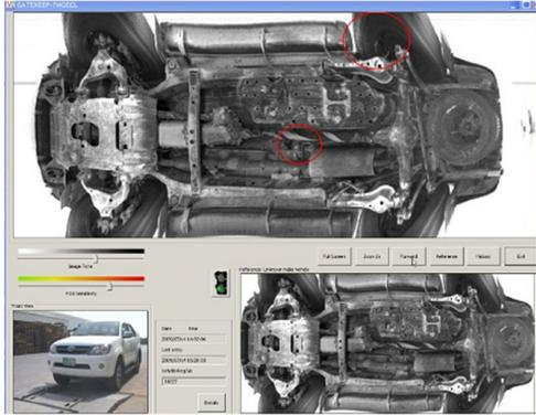
The operator screen may display the overview / driver image in colour. The undercarriage views are generally displayed in monochrome allowing for more pixel detail and thus better resolution than colour images. As computers analyze the image, monochrome is superior to colour.
