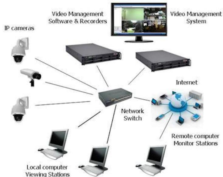
**The electronic security industry has moved into the IT space, with IP technologies growing in significance and application.** Most CCTV, access control, intruder detection and intercom systems now offer IP network interfaces, allowing devices or control panels to communicate over an IP infrastructure.
