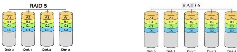
RAID is implemented either at the hardware or software level within a server or storage enclosure. For the performance needs of surveillance and truly enterprise class storage, a hardware RAID controller is a necessity for any surveillance video storage. Implementing RAID at the software level
