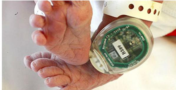
Radio Frequency Identification (RFID) Tags are fitted to a baby to accurately report Real-Time location and to avoid unauthorised removal of an infant from a ward. These RFID tags use the very latest in RFID Technology, transmitting a unique ID to the local network of readers to confirm the location of the baby.
