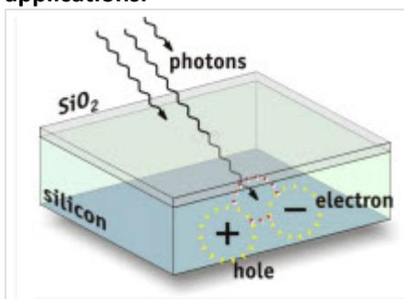
**Both CCD and CMOS image sensors depend on the photoelectric effect to create electrical signal from light. Both types of imagers convert light into electric charge and process it into electronic signals.**
