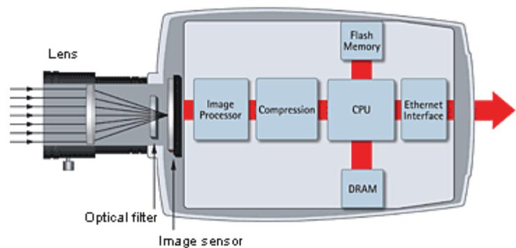
**There are two types of image sensors found in IP surveillance cameras - CMOS image sensors and CCD image sensors.**
