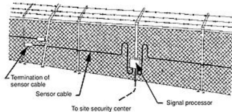
Strain-sensor cable installed on a chain-link/barbed-wire fence
