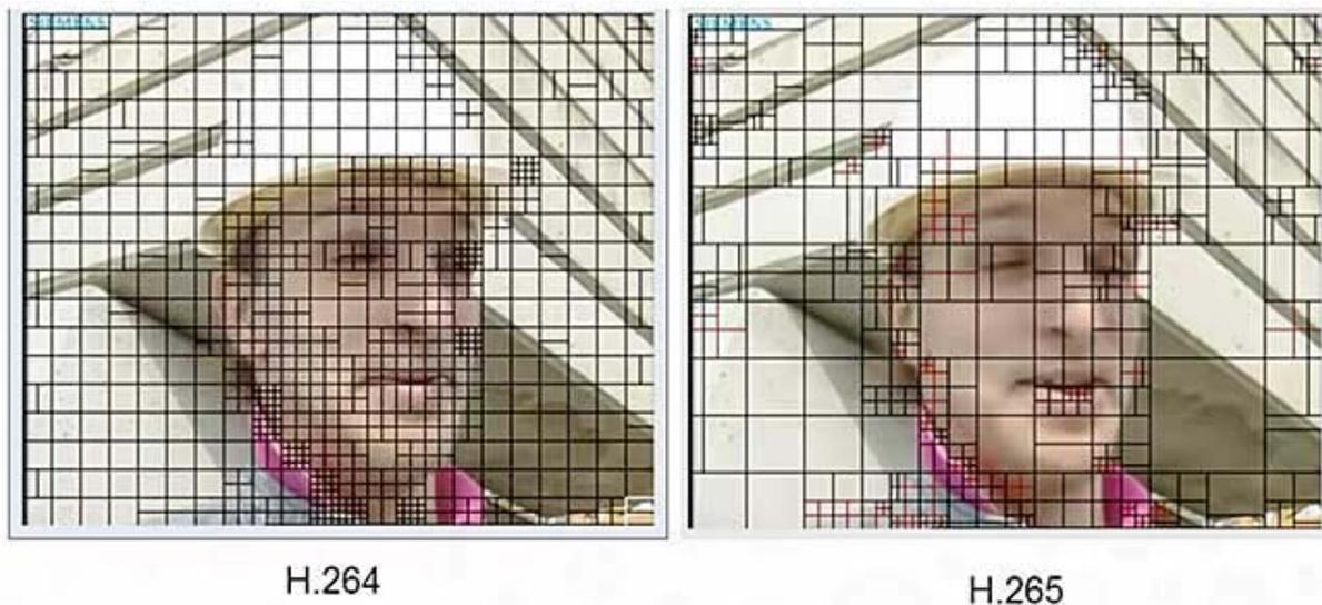
Where H.264 used 9 intra prediction directions, HEVC can use over 35, adding more potential reference pixel blocks that fuel more efficient intra-frame compression. The obvious cost is the additional encoding time required to search in the additional directions.
