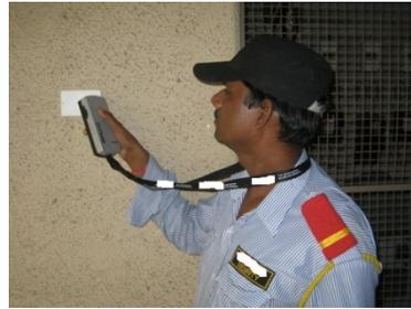
"Checkpoint stations" are used in place of key stations. These stations contain some type of device that can be read electronically and are used in place of the mechanical key. Depending on the manufacturer and type of system used, a barcode, magnetic strip, or memory button may be used in the checkpoint station. Like key stations, checkpoint stations are installed at various points along the desired patrol route.
