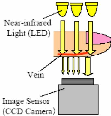
**Fig. 1 Capturing the finger vein pattern**
