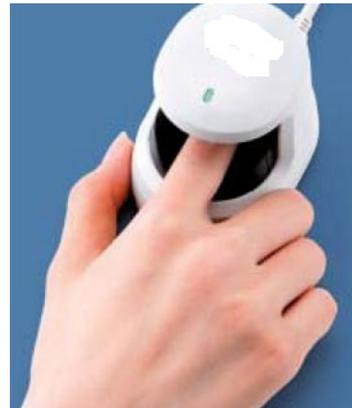
**Fig. 2 Typical finger vein reader**
