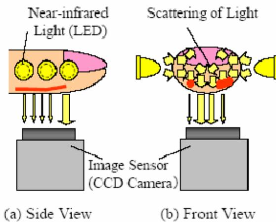
**Fig. 3 The side-illumination technique**
