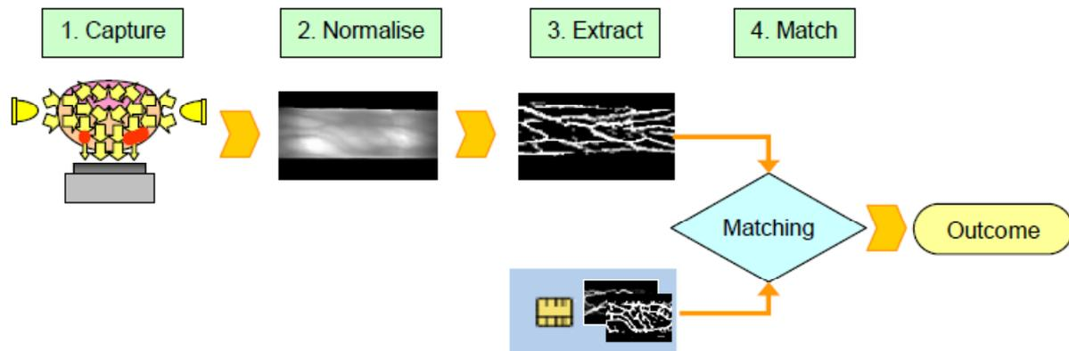
**Figure 5 Block diagram of finger vein authentication**
