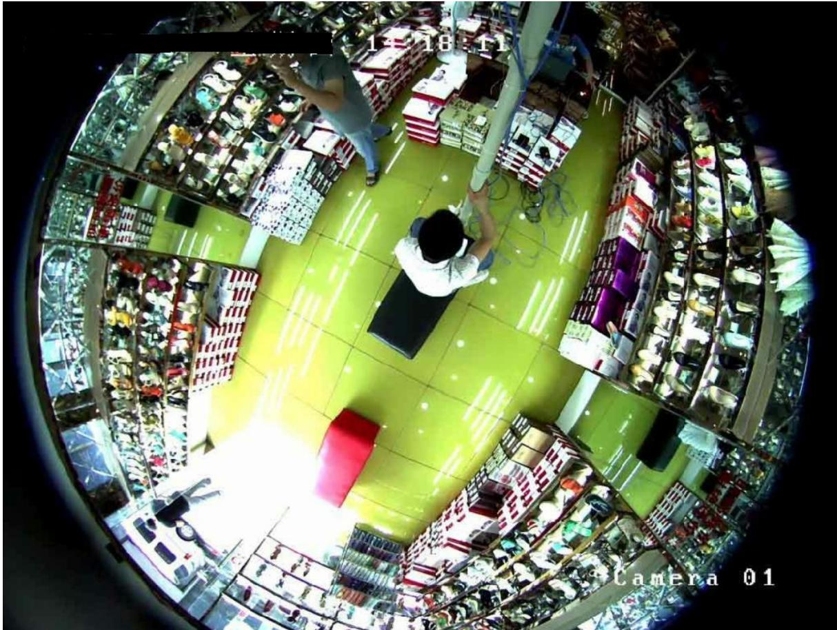
**Fisheye and panoramic cameras offer a 360 degree field of view.** Unlike fixed cameras that narrow in on a specific spot or area, fisheye and panoramic cameras can cover a much wider area. A fisheye or panoramic camera can provide surveillance for broad areas like stores, warehouses, parking lots, stadiums, museums, concert halls, and ports.
